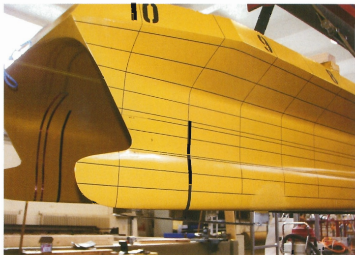
Above: a hull model for the ShadowCAT ready for testing
